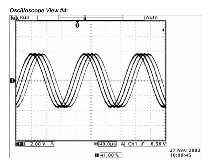
The waveform is sliding sideways across the screen and does not stay in one place. Look at the oscilloscope settings and identify what is causing the rolling display.
