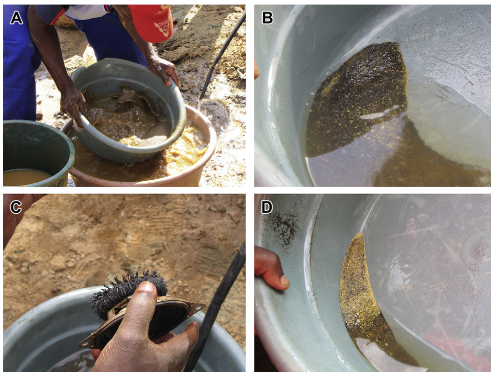
Fig. 3. Gold separation using magnets. (A) Ore from the connecting pipe and centrifuge is collected and panned. (B) Sediment containing gold and iron. (C) A speaker magnet is used to remove iron and magnetic species. (D) After separation, mostly gold remains.
