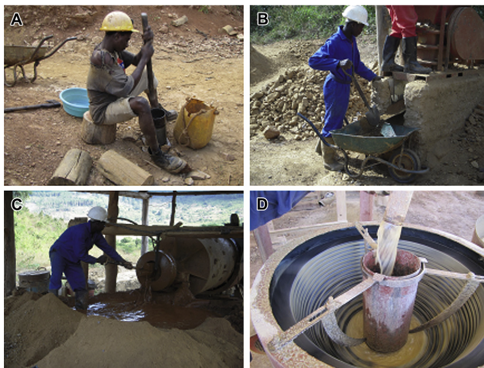
Fig. 2. Clean Tech Mining Practices. (A) Manual crushing of ore with mortar and pestle. (B) Grinding rough ore into small fragments. (C) Crushing ore with an industrial ball mill. (D) Centrifuge basin for collecting gold particles.
