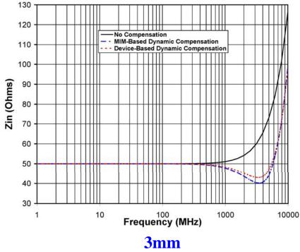
Worst Case : 5mm $f_{+/-10\%}$  No Dynamic Capacitance =1.9 GHz $f_{+/-10\%}$  w/ Dynamic Capacitance =4.1 GHz
